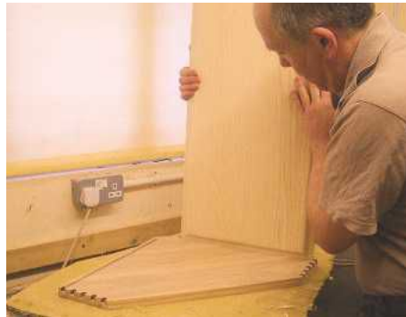
▲ Pic.11 Check the fit of a panel in the routed grooves. Remember that the finish will increase the thickness marginally
